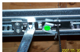
Figure 1: Carriage is engaged
